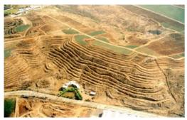
The graded bunds, commonly used are comparable to the narrow base terraces. They are used for the safe disposal of excess runoff in high rainfall areas and regions where the soil is relatively impervious [clay]. Farming operations are not done on bunds or bund channels. *Function:*
